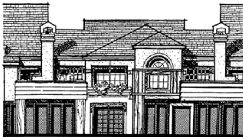
Articulated facade gives appearance of a collection of smaller structures
