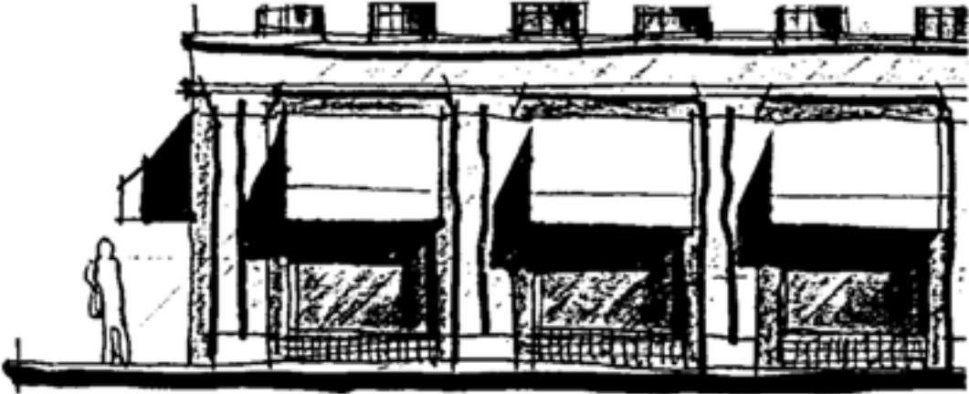
Shed Awning At Lower Level Is Consistent With Rectilinear Building Form.
