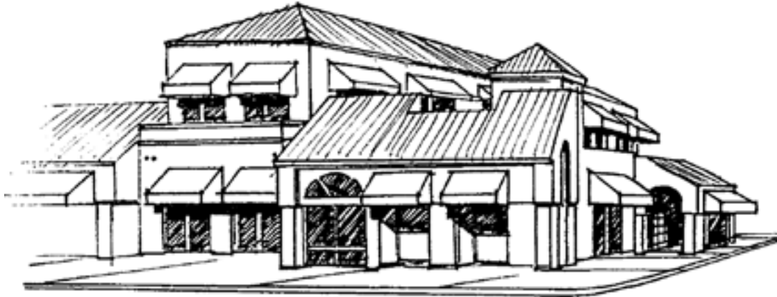
AWNINGS OF THE SAME FORM AND LOCATION ARE REPEATED, WITH THE SIGNAGE ON THE AWNING'S VALANCE.
